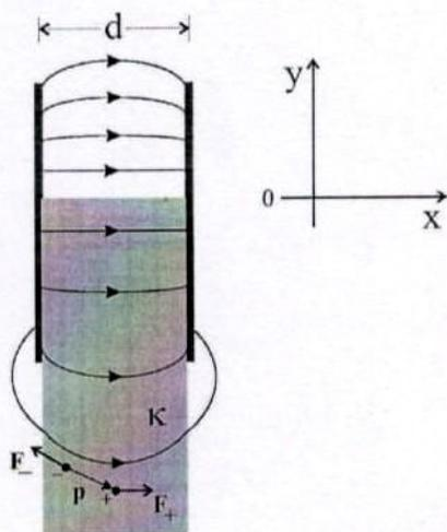
Fig. 1. Linear dielectric slab partially inserted between parallel conducting charged plates. Unbalanced forces  $F_+$  and  $F_-$  are shown acting on a dipole  $p$  in the fringing field region. The  $+z$  direction is out of the page.
