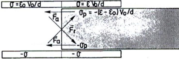
Fig. 2. The charge on the density on the upper conducting surface is  $\sigma = \epsilon_0 V_0 / d$ , which produces an attractive force  $F_a$  on the charge  $\sigma_p = -(\epsilon - \epsilon_0) V_0 / d$  on the upper dielectric surface; and a repulsive force  $F_r$  on the charge  $-\sigma_p$  on the lower dielectric surface.
