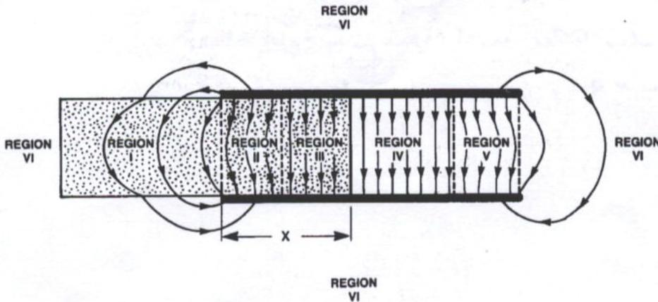
Fig. 3. Division of all space into six regions for the purpose of evaluating the total field energy. Regions I, II, and III are within the dielectric; regions IV, V, and VI are in vacuum.
