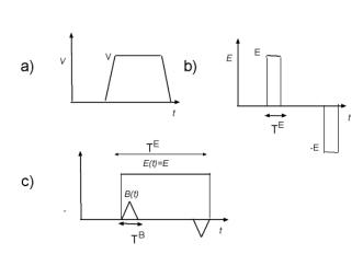
Figure 3.4: Constant voltage pulse (a) and the corresponding electric (b) and magnetic (c) pulses in the bi-filar coil.
