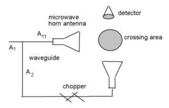
Figure 8.2: Schematic representation of the experimental arrangement of Ranfagni and collaborators discussed in [16].
