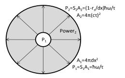
Figure 3 Poynting Vector between inner cutoff and distant outer boundary
