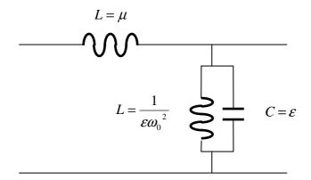
The line is dispersive because the characteristic impedance (38) is not constant but depends on the frequency. The line resonates to:
