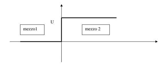
Formula (140) for  $k_z$  allows the calculation of speed in medium 2 and therefore also allows an analogy with the propagation of TE in a waveguide 2 with a different cutoff frequency (or size  $d_2$ ).
