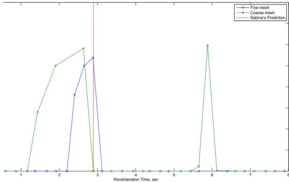
FIG. 4. Effect of refinement of the finite element mesh on the mode fraction distribution.
