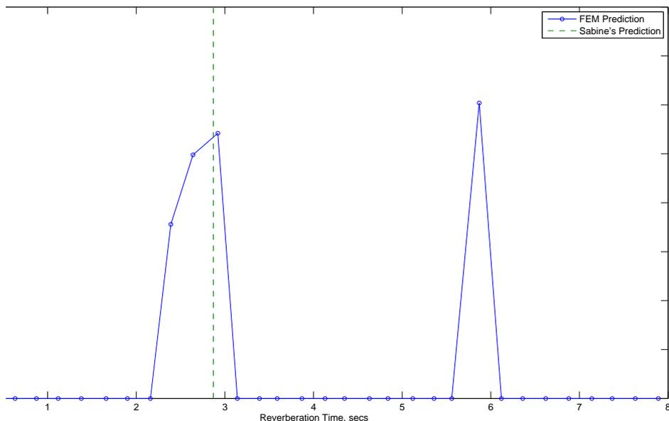
FIG. 2. Mode fraction distribution as a function of the reverberation time, for a rectangular room of dimensions  $4m \times 5m \times 6m$  having lining distributed uniformly on one of the x-walls.
