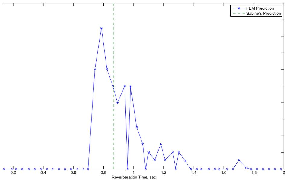
FIG. 7. Mode fraction distribution as a function of the reverberation time, for a rectangular room of dimensions 4 m x 5 m x 6 m having absorptive lining distributed uniformly on three orthogonal walls.
