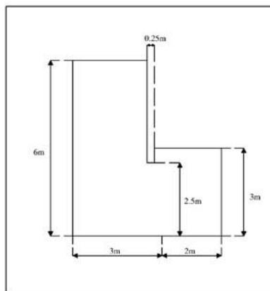
Fig. 25. Elevation view of a simple coupled room
