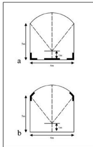
FIG. 5. Cross-sectional view of a room with a barreled ceiling. The ceiling is covered with absorptive material and the dark patches indicate effective positions for placing patches of absorptive material (a). Cross-sectional view of a room with a barreled ceiling. The floor is covered with absorptive material and the dark patches indicate effective positions for placing patches of absorptive material (b).
