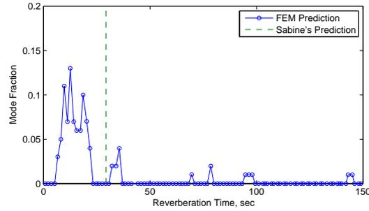
FIG. 8. Mode fraction distribution as a function of the reverberation time, for a rectangular room of dimensions 4 m x 5 m x 6 m having absorptive patch at one of its corners.
