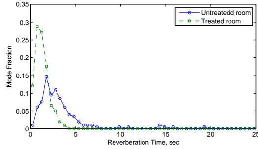
FIG. 11. Effect of treating the room of configuration with absorptive patches, on the reverberation time
