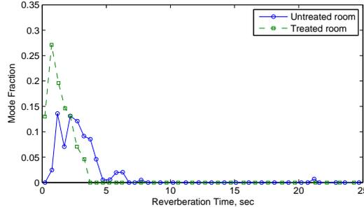
FIG. 10. Effect of treating the room of configuration of Fig. 17 with absorptive patches, on the reverberation time.
