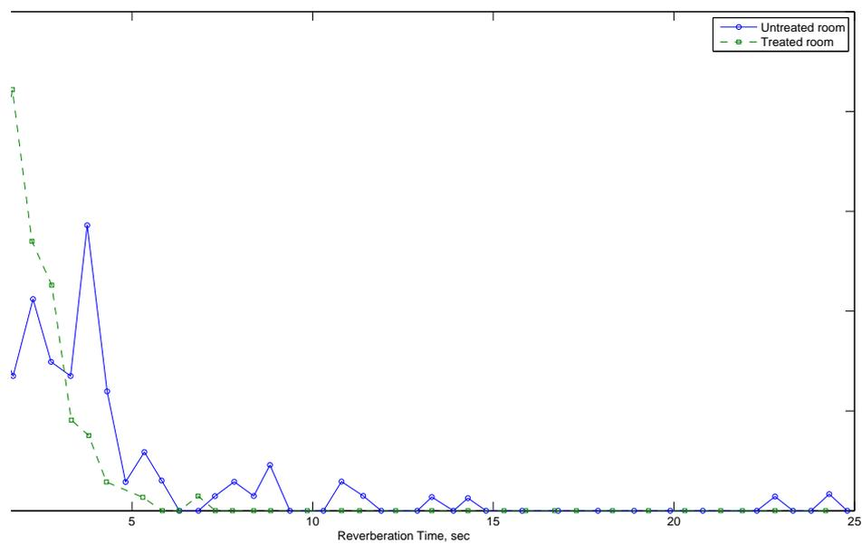
FIG. 9. Effect of treating the room of configuration of Fig. 5(a) with absorptive patches, on the reverberation time.
