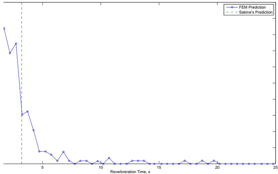
FIG. 16. Mode fraction distribution as a function of the reverberation time for the coupled room of configuration shown in Fig. 25.
