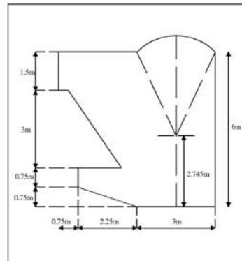
Fig. 23. cross-sectional view of a showing the elevation of a slightly complex Auditorium. The dark patches indicate locations where placing of absorptive lining would dampen the modes having long reverberation times.
