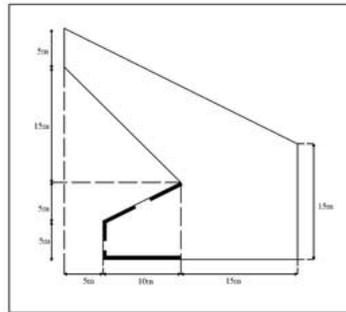
FIG. 12. Cross-sectional view showing the elevation of a simple Auditorium. The dark patches indicate locations where placing of absorptive lining would dampen the modes having long reverberation times.
