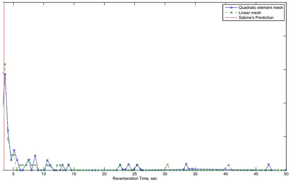
FIG. 6. Effect of using linear and quadratic elements on the mode fraction distribution.
