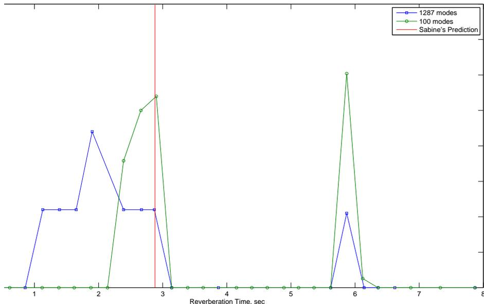
FIG. 3. Effect of the number of modes on the mode fraction distribution.
