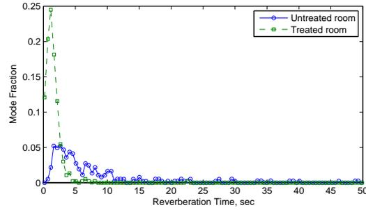
FIG. 14. Effect of treating the room of configuration with absorptive patches, on the reverberation time.
