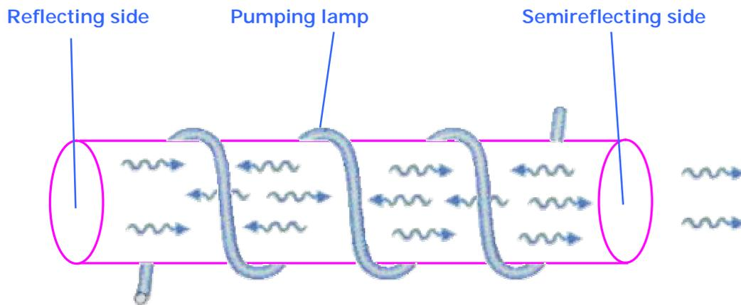
The ruby Laser is the first kind of Laser ever built; the ruby is a corundum crystal ( $Al_2O_3$ ) with impurities of ions  $Cr^{+++}$ . Ruby has got a strong absorption band in the green and it's used to make the inversion of population.
