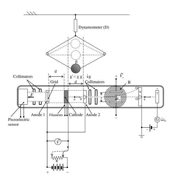
Fig. III – Experimental set-up in order to check the factor  $\chi$  above a high-speed electrons flux. The set-up may also check the velocities and the gravitational masses of the electrons.
