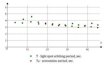
**Fig. 9.** Dependency of the light spot orbiting period and the gyroscope precession period on time
