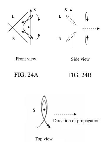
Intrinsic spin for a propagating positively charged particle. Note that (S) is out of the page using the right hand rule.
