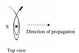
Intrinsic spin for a propagating negatively charged particle. Note that (S) is into the page using the right hand rule.
