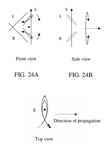
Intrinsic spin for a propagating positively charged particle. Note that (S) is out of the page using the right hand rule.
