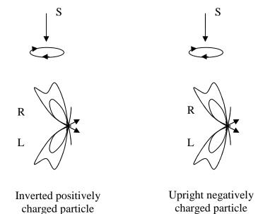
Juxtaposed positively and negatively charged particles propagating in parallel out of the page
