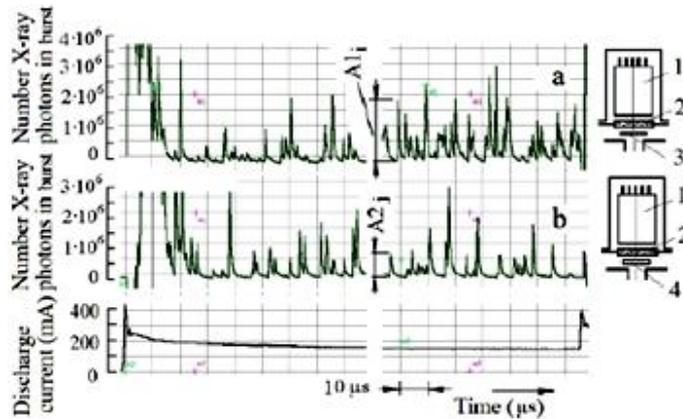
**Figure 6.** Typical oscillograms of X-ray emission from the PMMA/PM scintillator detector covered with Be foils with different thicknesses: (a) covered with a 15  $\mu\text{m}$  Be foil; (b) covered with a 30  $\mu\text{m}$  Be foil. In this case the cathode was Pd, the gas was  $\text{D}_2$ , and the discharge current was 150 mA.
