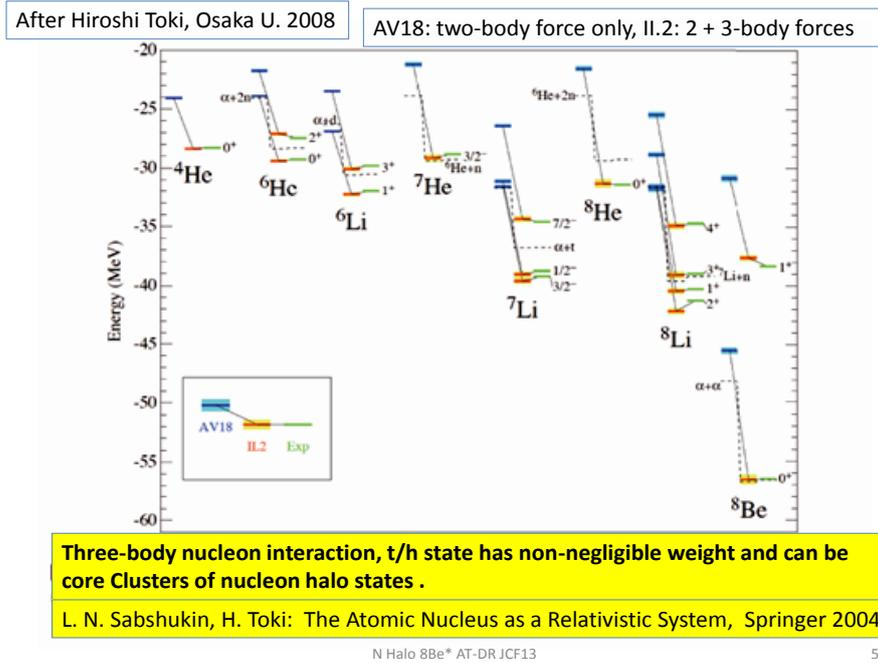
Fig.3: Nuclear binding energy calculated for light nuclei [4]
