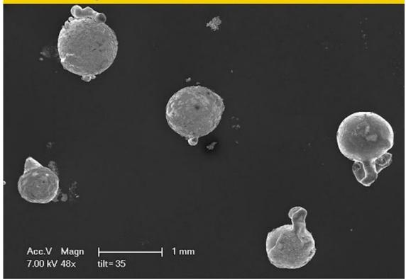
Figure 1, Image of some silicon nuclei, all with globular shape and equipped with one large and several smaller appendices and diameters between 0.4 and 0.8 mm
