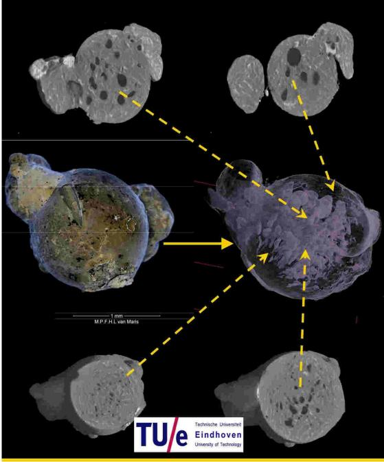
Figure 10, Internal Silicon globule structure made by 2D and 3D Nano CT scan at the University of Eindhoven (NL) Internal roughly linear cone shaped hollow bullet energy tunneling channels are observed, in black color at the 4x cross sections.
