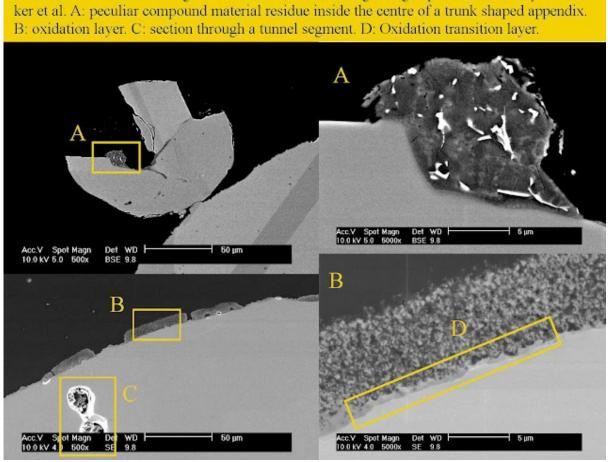
Sectional view of a Silicon globule of the Silicon Ball Lightning experiment made by R. Dek-
