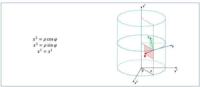
Figure 1. Axially symmetric field configuration
