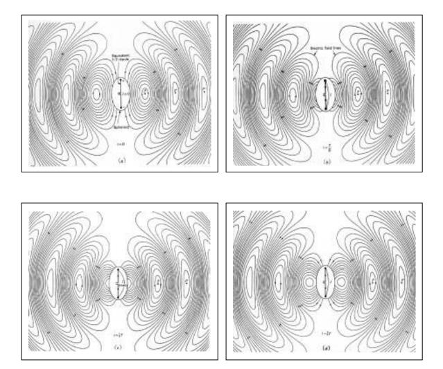
Five stages of radiation from a dipole antenna are shown in
