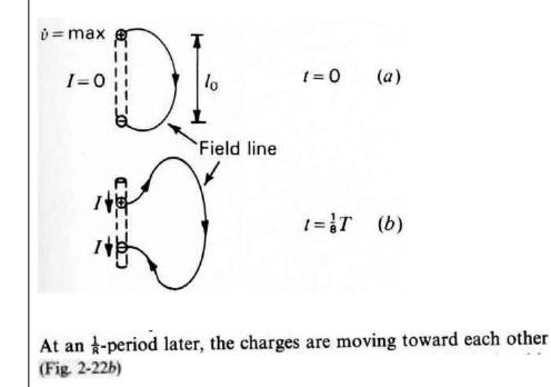
By comparing the field lines in figures (a) and (b), observe that the author claims, *without bringing any evidence to support his statement*, that the field line lags behind the moving charges and that the *field line moves on its own further away* from the charges producing it.
