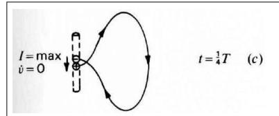
and at a  $\frac{1}{4}$ -period they pass at the midpoint (Fig. 2-22c). As this happens, the field lines detach and new ones of opposite sign are formed. At this time the equivalent current I is a maximum and the charge acceleration is zero.
