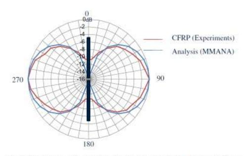
Fig. 8. Experimental and analytical two-dimensional radiation patterns of dipole antennas using the CFRP rectangular specimens. The analytical pattern was obtained using the antenna simulation software MMANA.
