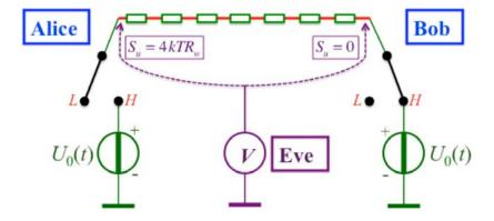
Figure 7. The BR scheme with finite wire resistance and the Johnson noise attack.
