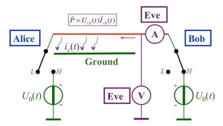
Figure 5. Universal, energy-flow-analysis-attack against the BR scheme (even in the no-wave transient limit provided by proper voltage time functions by eliminating high-frequency components). The direction of power flow, energy flow or that of the current fully characterizes the situation for Eve. Similarly the size of power flow, energy flow and current flow versus location also fully compromise the security.
