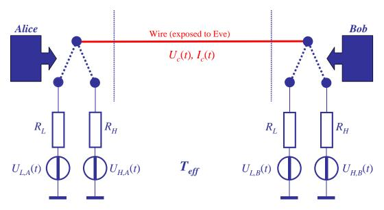
Fig. 1. Outline of the core KLJN system. Parasitic elements leading to non-ideal features and defense circuit block (current/voltage monitoring/comparison) against invasive attack are not shown/discussed here.
