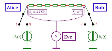
Figure 7. BR's scheme with finite wire resistance and the Johnson noise attack. With  $R_w$  wire resistance, in the steady-state mode, Eve will measure zero power density spectrum  $S_u$  at the closed end and  $S_u = 4kTR_w$  at the open end.
