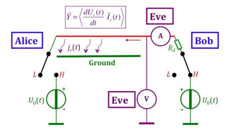
Figure 6. Transient-damping resistor version of BR's scheme, and capacitive noise current attack. The direction and the location-dependent value of the cross-correlation vector  $\vec{Y}$  of the time-derivative of the channel voltage and the current vector provide two ways to crack the key while the location-dependence of the RMS channel current offers a third way.
