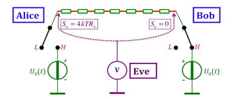
Figure 7. BR's scheme with finite wire resistance and Johnson noise attack. With a wire resistance of  $R_w$  and in the steady-state mode, Eve will measure zero power density spectrum  $S_u$  at the closed end of the wire and  $S_u = 4kTR_w$  at the open end.
