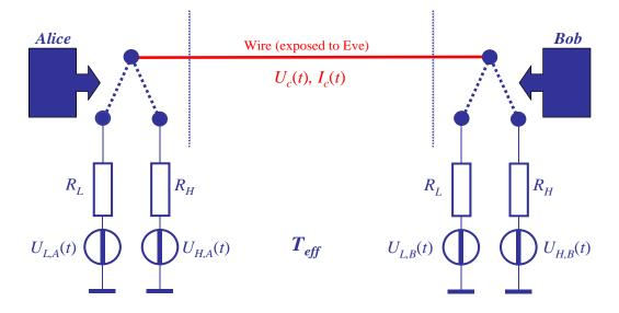
Figure 1. Outline of the core KLJN key exchange system. The communicator parties, Alice and Bob, randomly choose and connect either  $R_L$  or  $R_H$  to the wire. The (effective) temperature  $T_{eff}$  is publicly agreed and kept, and the (enhanced or standard) Johnson noises of the resistors  $U_{LA}(t)$ ,  $U_{LB}(t)$ ,  $U_{HA}(t)$ , and  $U_{HB}(t)$  are independent
