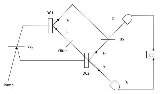
Figure 1 The ZWM : Two downconversion crystals (DC1 & 2) are commonly pumped. Their outputs, signal and idler photons labelled s and i, are arranged so that  $i_1$  transmits through DC2 and comes into exact alignment with  $i_2$ . The combination of  $s_1$  and  $s_2$  only results in interference when the idler  $i_1$  is not attenuated at the filter.
