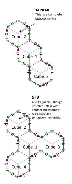
Figure 7: Acceptable forms of COMPLETE subassemblies.
