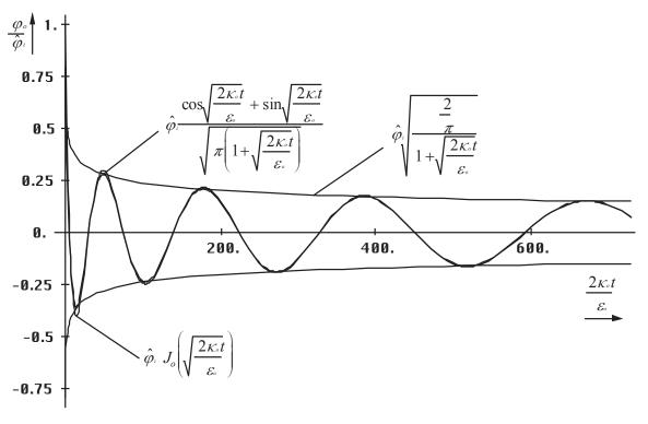
Figure 13 Course of magnetic flux as well as of approximationand envelope-function (127) during a longer time period
