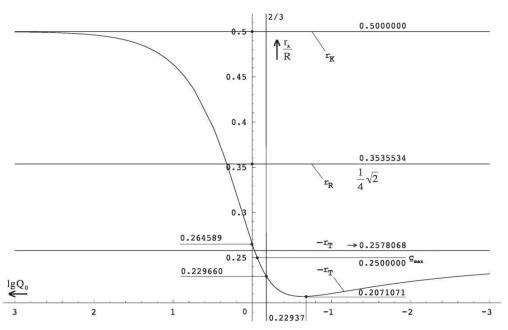
$\begin{array}{c} Figure~145\\ Course~of~the~distance-vectors~r_{R},~r_{K}~and~r_{T}\\ at~the~SCHWARZSCHILD-radius~\left(Q_{0}{=}10^{0}\right) \end{array}$
