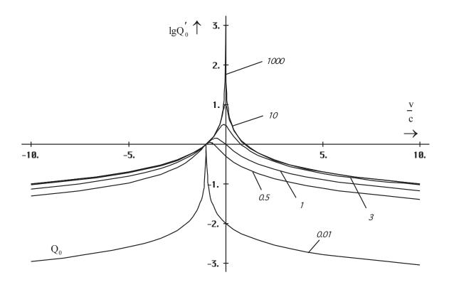
Figure 129 Course of the Q-factor being relevant for the system S´ with respect to the velocity in reference to the system S (metrics) for  $Q_0 \le 10^3$ .
