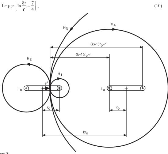
Figure 3 Magnetic field-strength in one and in several conductor loops
