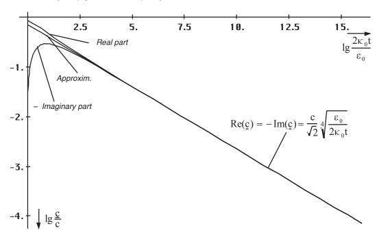
Figure 29 Propagation-velocity in dependence of time (logarithmic)
