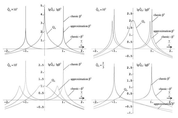
Figure 103 Relativistic dilatation-factor  $\beta$  and Q-factor as a function of the velocity
