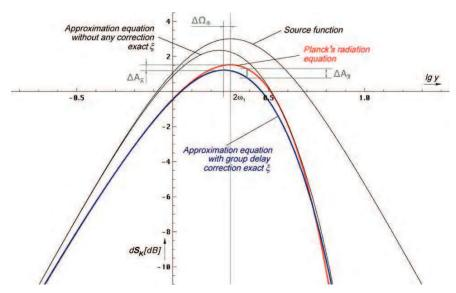
Figure 10 PLANCK's radiation-rule and approximation with group delay correction under application of the exact function  $\boldsymbol{\xi}$  (relative level) high resolution
