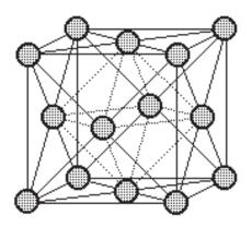
Figure 1 Cubic face-centered crystal lattice
