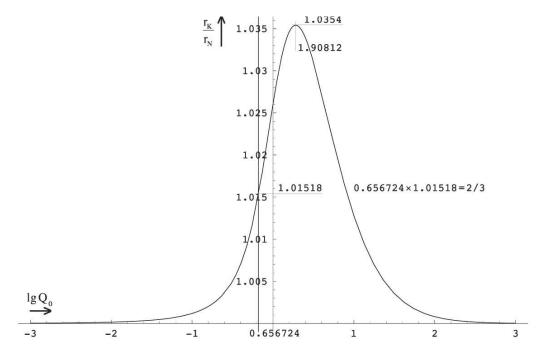
Figure 116 Ratio between the length of the constant wave-count vector  $r\kappa$  and the length of the zero vector  $r\kappa$  as a function of  $Q_0$
