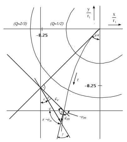
Figure 98 Vectorial speed-addition with neutrinos near the singularity
