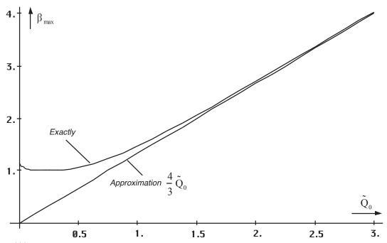
Figure 111 Exact course and approximation for the maximum super elevation  $\boldsymbol{\beta}$  at the time- and space-like photon
