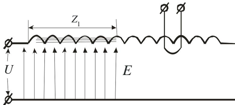
Fig. 5. The diagram of the propagation of magnetic and electrical pour on in the long solenoid.
