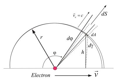
Figure 13: Emitted Energy flux density dS of a moving electron
