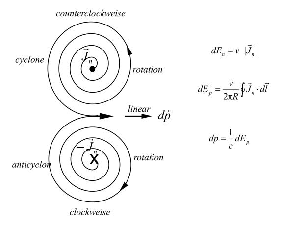
Figure 5: Generation of linear momentum out of opposed angular momenta
