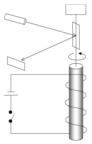
Figure 2.2: The experiment to verify the angular momentum of the spin
