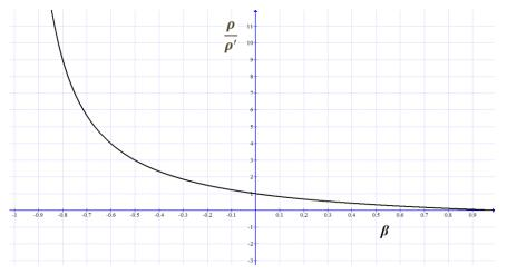
Figure a5. Mass density as a function of velocity
