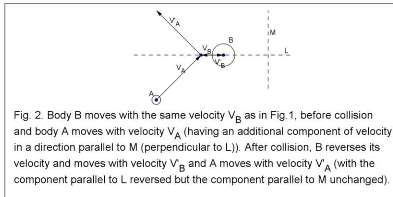
After the collision, B moves away with velocity  $\mathbf{V}'_B (= -\mathbf{V}_B)$ . Body A moves away with its velocity component parallel to L reversed, and the velocity component perpendicular to L unchanged, obeying the law of conservation of momentum. It moves away with velocity  $\mathbf{V}'_A$ .
