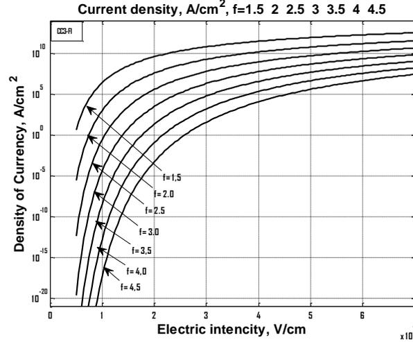
**Fig.6.** Density of electric currency the noodle injector via the electric intensity for different the field electron emissions  $f$ .
