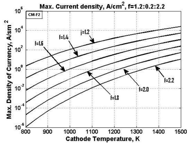
**Fig.5.** The maximal electric current via cathode temperature for the different exit work of electrons  $f$ .
