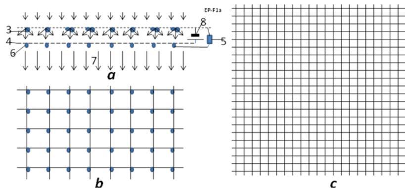
**Fig.2.** Electron ramjet engine (ABEP) for vertical start. *a* – side view, *b* – net of injector (top view), *c* – lower electrode (lower view). *Notations:* 3 – injector of charges (forward electrode), 4 – back electrode, 5 separator of charges; 6 – lower injector of charges (opposed the forward injector 3), 7 – air flow. 8 – source of high voltage (example, the electrostatic generator).
