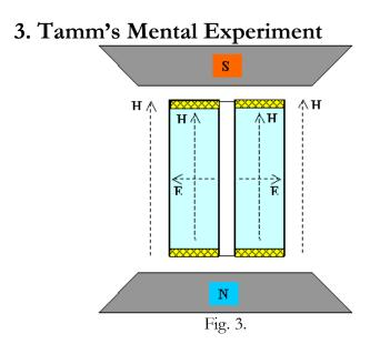
In [4] Tamm describes the following mental experiment – see Fig. 3. He considers a cylindrical capacitor placed in a uniform magnetic field **H**, parallel to its axis. In the space between the capacitor plates, in addition to the magnetic field, there is also a radial electric field of intensity **E**, created by the charged capacitor. In the space between the capacitor plates in the static electromagnetic field there exists the
