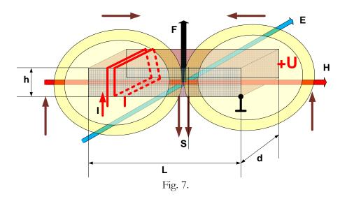
Let us discuss in detail the calculation of force (1), using the notations of the body dimensions shown in the Fig. 7 ure: L, d, h. We have:
