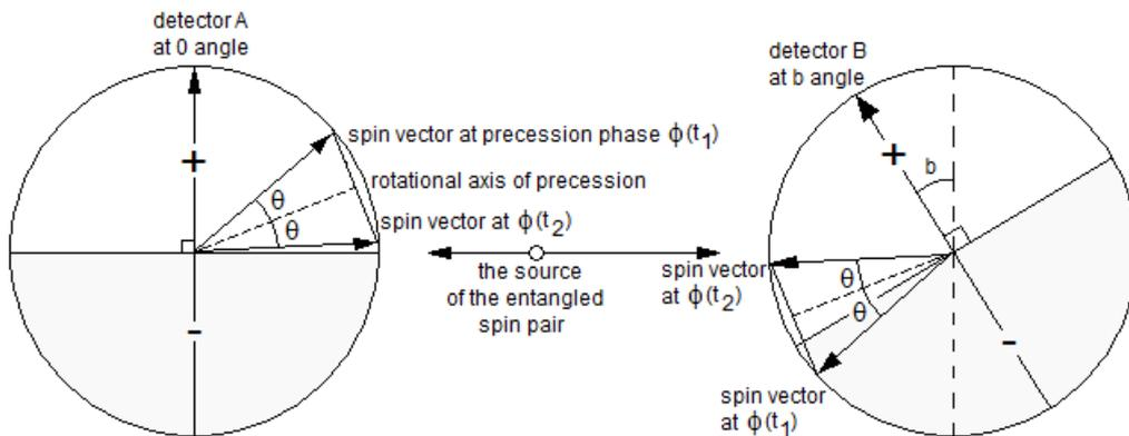
Figure 2: Detection of two anti-parallel spin particles with precession
