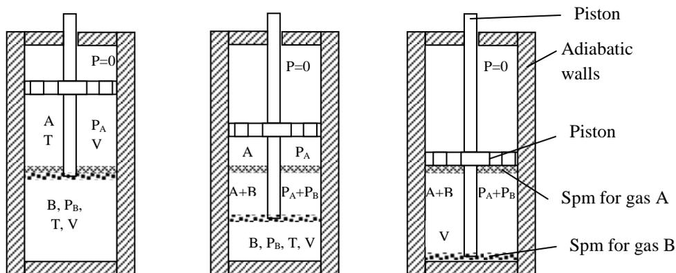
FIG 1.1 Reversible mixing of two ideal gases A and B with two semipermeable membranes
