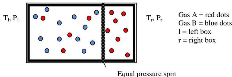
Fig 2.1 Gas A is separated from the mixture at the right box and has pressure equal to the total pressure at the left box
