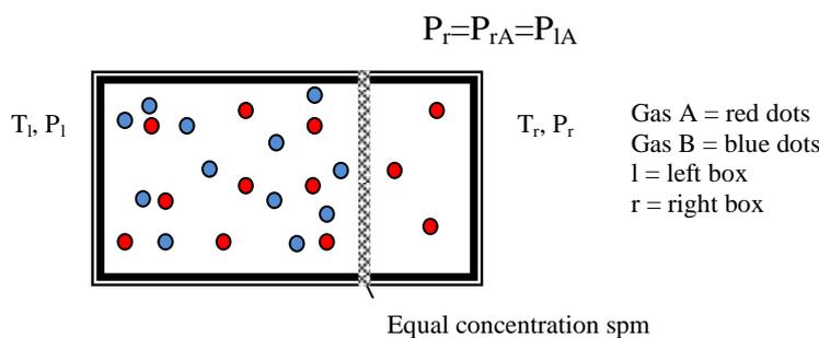
Fig 2.2 Gas A is separated from the mixture at the right box and has pressure equal to it partial pressure at the left box
