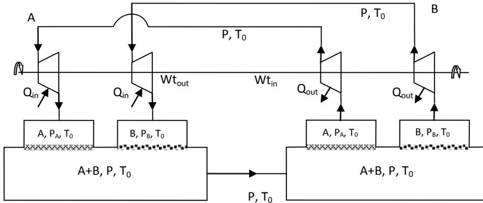
FIG 1.2 Mixing & separation of two ideal gases “reversibly” in a closed loop
