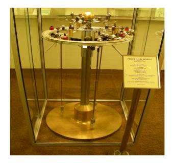
A similar machine, called "Perpetuum Mobile" has long been functioning in Helsinki Science Museum. In 1990 its bearings were replaced and it continued to work.
