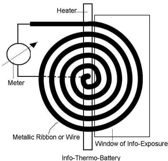
Fig.18. Info-Thermo-Battery as a sensor of exposure to information. Action of information on a metal can be multiplied by a series connection of the metal elements, working like connected in series thermocouples at the heating.
