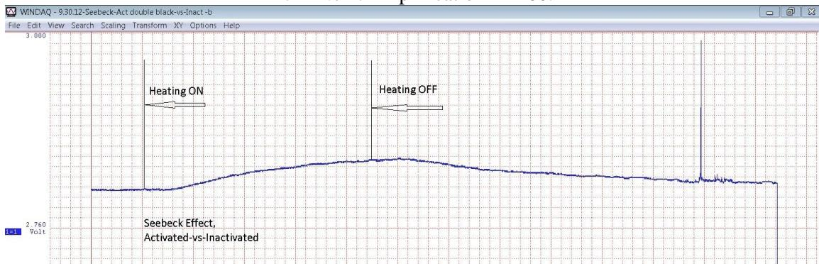
Fig.9. Amplified thermo-EMF of a pair composed of activated-non-activated aluminum matrixes.
