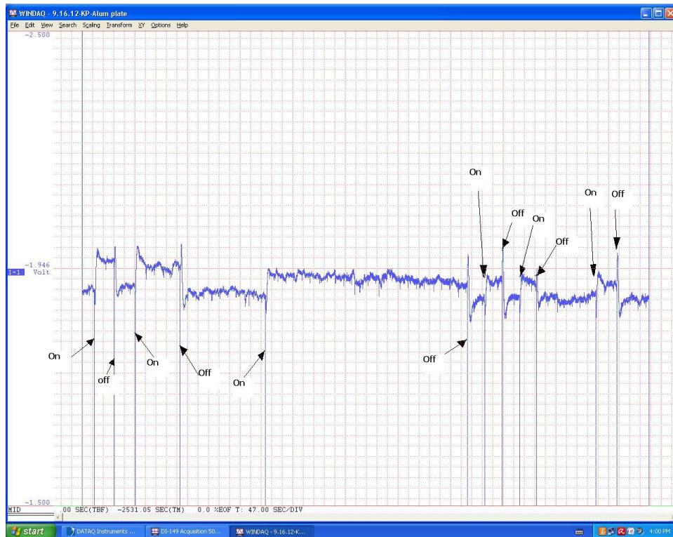
Fig.11. Aluminum plate (no activation), 133 mV. The spikes on the record are caused by inertia of the electromagnet, vibrating the copper reference.
