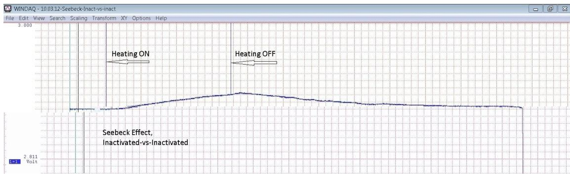
Fig.8. Amplified thermo-EMF of two aluminum matrixes with no info-activation.
