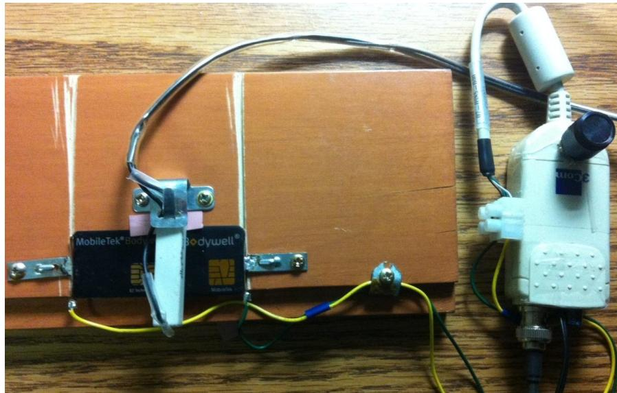
Fig.5. Experimental installation for comparing the work function of two samples of metals basing on Seebeck effect. Under heating they work as a thermocouple. The ceramic heater is placed over a joint of the samples. The unit on the right amplifies the signal.
