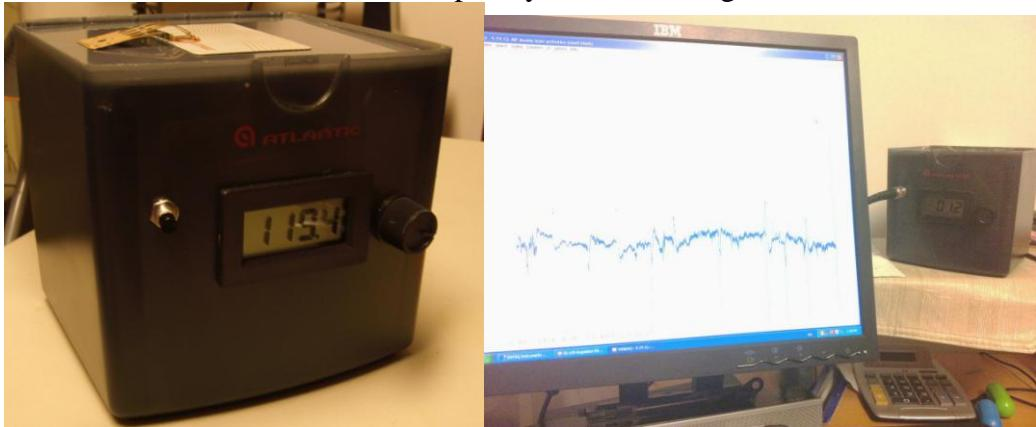
Fig.7. Kelvin Probe used for the experiment was developed by the author. The samples were placed on the upper platform having a contacting electrode. There was a vibrating copper plate under the platform. The processed signal entered the computer recorder DATAQ.
