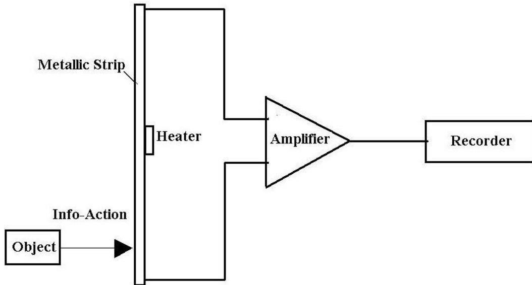
Fig.6. Modification of the installation of Figs. 2 and 3 for detecting influence of info-injection on the work function of metals basing on the Seebeck effect. The info-action changes properties of the foil/strip that converts the upper and lower portions into a thermocouple when the heat is applied at the centre.
