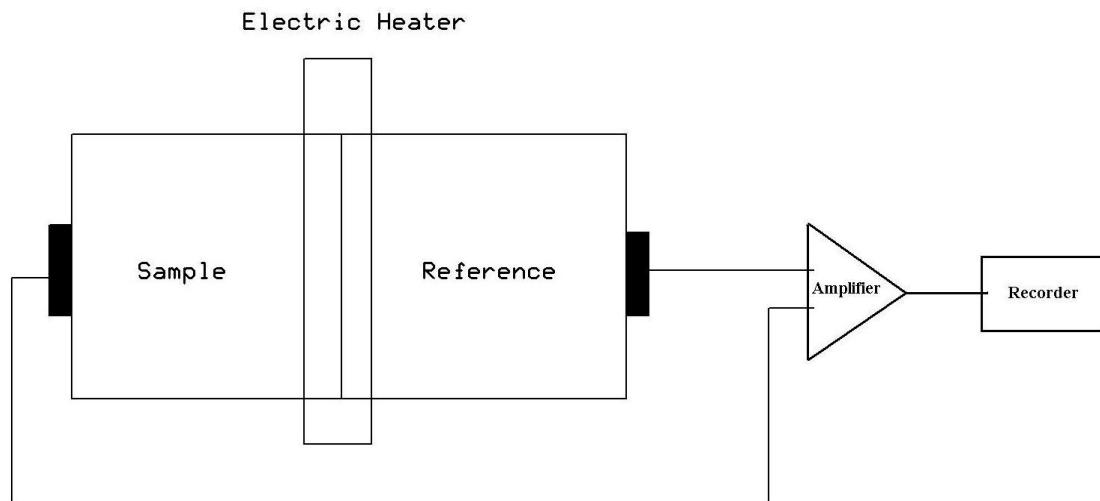
Fig.4. Conception of comparing work functions of two samples of metals basing on Seebeck effect. Being heated at the joint, the system works as a thermocouple if the work functions are not equal.
