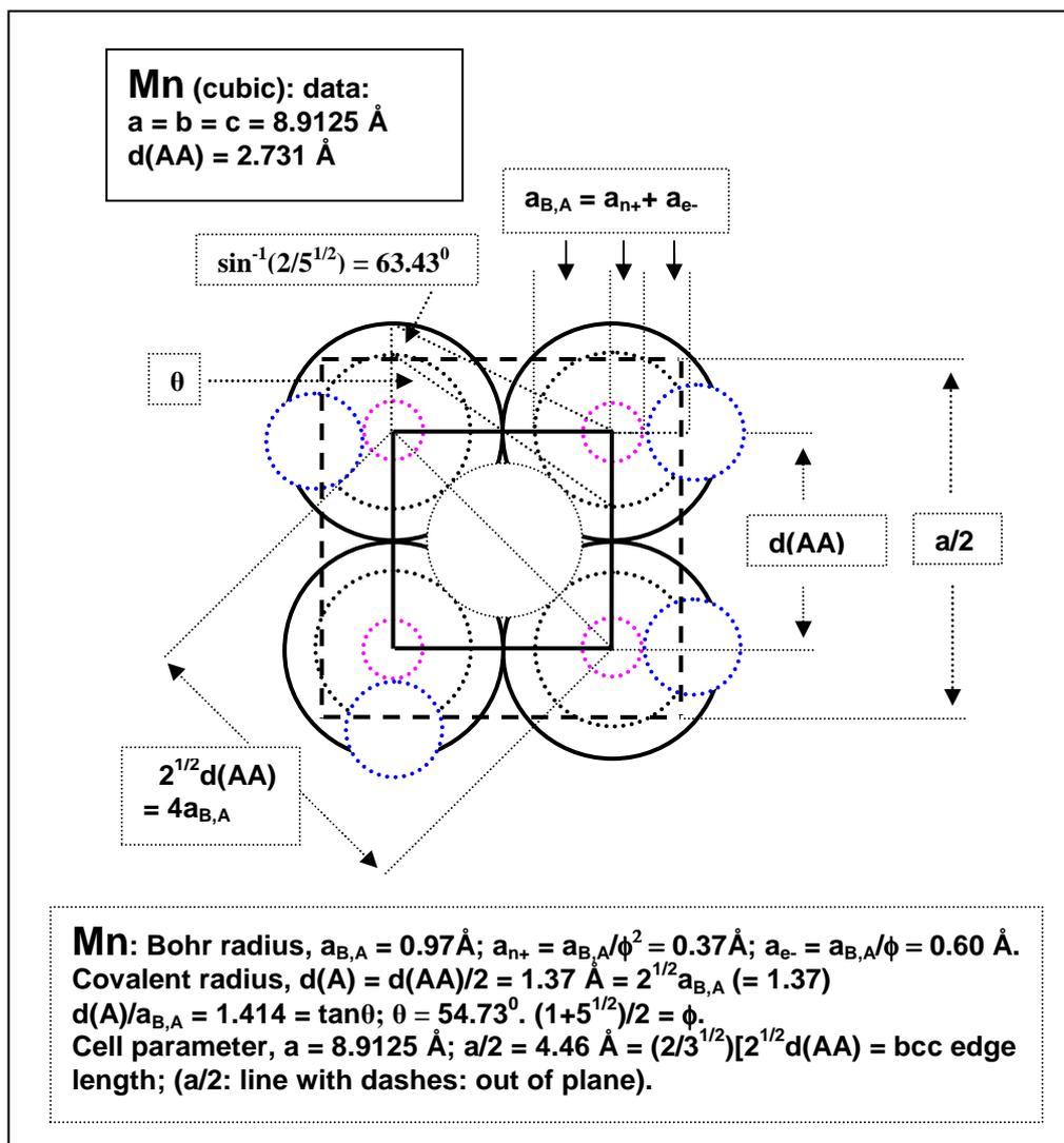
Fig. 3. Structure at the atomic level of Manganese. The cell parameter,  $a = b = c = 8.9125 \text{ \AA}$ . The distance  $a/2$  is of a body center cube with the center to edge distance equal to  $2^{1/2}d(\text{Mn-Mn})$ , which is the diagonal of the square with sides equal to  $d(\text{Mn-Mn})$ .  $a_{\text{B,A}}$  is the Bohr radius and  $a_{\text{n}^+}$  and  $a_{\text{e}^-}$  are the radii of its nucleus and electron.
