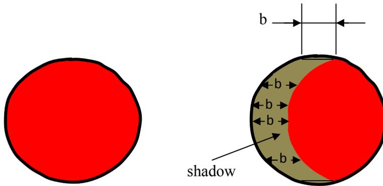
The left diagram shows a bright circular spot on the photo diode which will occur when there is no bending of the light ray. The right diagram shows what the spot of the light ray on the photo diode looks like, with a shadow due to bending of the light ray. Note that the size of the shadow has been exaggerated, which is actually only about 16.56% of the total area of the circle for an absolute velocity of 390 Km/s of the Earth.
