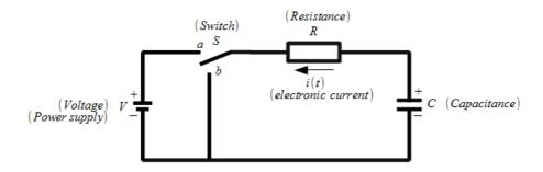
**FIGURE 1:** *RC* Circuit. When the switch S is open (position b) there is no current through the circuit. When the switch is closed (position a) a current *i* flows through the circuit and the capacitor *C* will get charged according to an exponential function. The time constant of the circuit is *RC* (*Resistance* times *Capacitance*). Note that the direction of the current is the actual direction of the electrons in the circuit.
