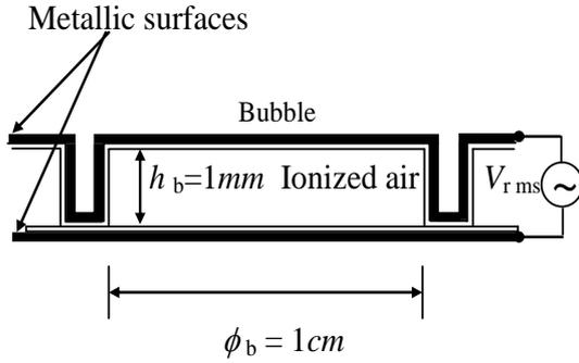
Fig.5 – Dimensions of the bubbles
