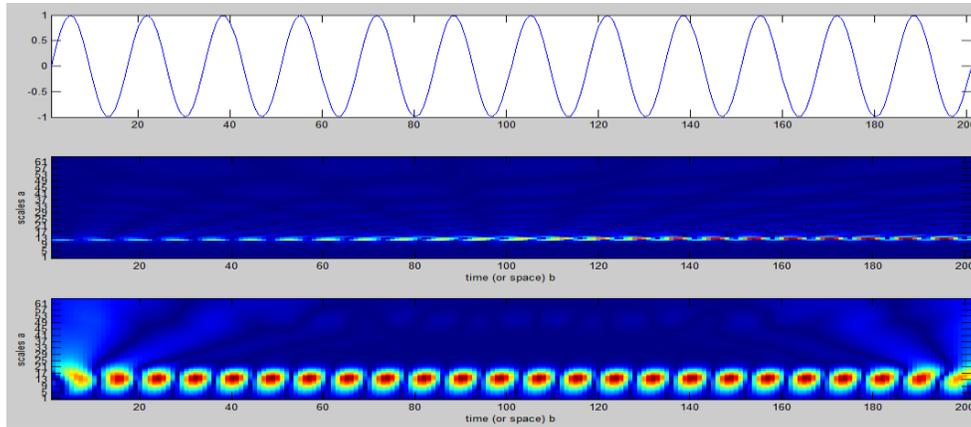
**Figure 3 Solitary Chirplet (above) and Wavelet (below) analysis of a Sinusoidal Signal**
