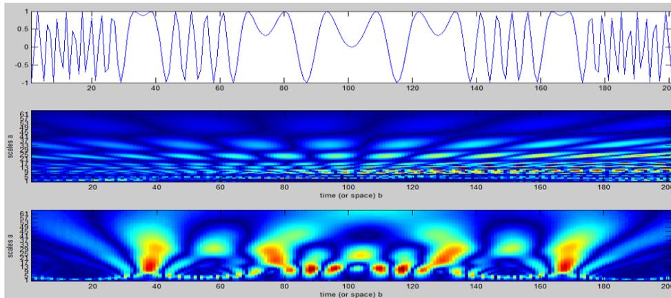
Figure 4 Solitary Chirplet (above) and Wavelet (below) analysis of a Frequency Modulated Signal
