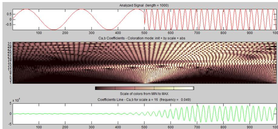
Figure 5 Solitary Chirplet analysis of a Signal with Discontinuity in frequency
