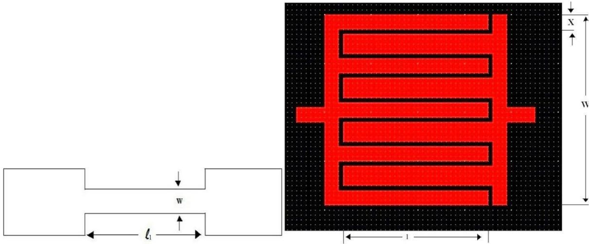
Figure 2 Structure of Inductor (left) and Capacitor (right)
