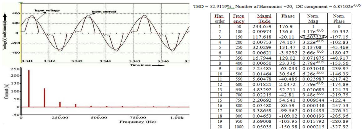
Figure 3 Waveform, Spectrum and THD analysis of diode bridge rectifier without filter
