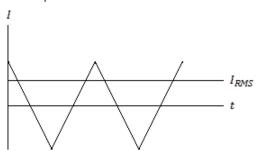
**B.** Waveform and root mean square (RMS) value of the output coil current
