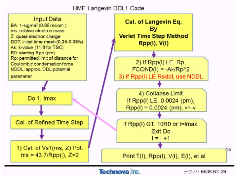
Fig.9: Flow chart of HME Langevin DDL code
