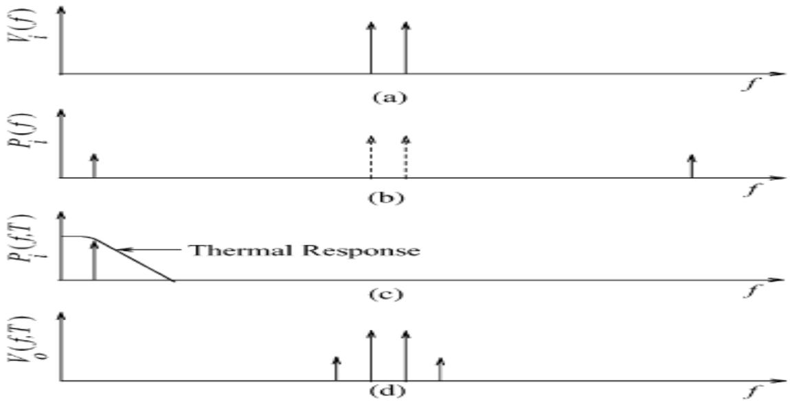
Fig. 1. Passive mixing process inherent in coupled electrical and thermal systems with: (a) input spectrum of voltages  $V_i(f)$  resulting from two-tone excitation, (b) input power spectrum  $P_i(f)$  resulting from a two-tone excitation, (c) component of the input power spectrum  $P_i(f, T)$  at baseband able to interact with the thermal response, and (d) output spectrum of voltages  $V_o(f, T)$  after electro-thermal mixing has occurred.
