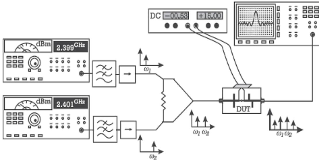
Most commonly used two-tone test measurement setup.
