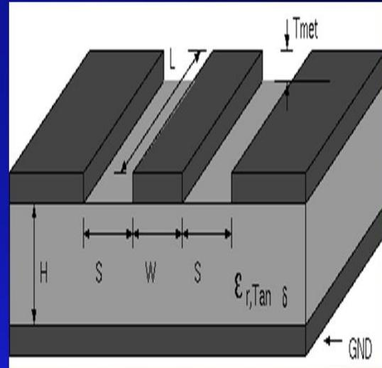
Figure 25 Model parameters of Gold Coplanar Waveguide
