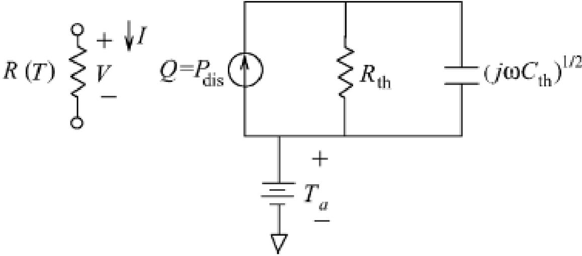
Figure 16 Equivalent circuit of resistor
