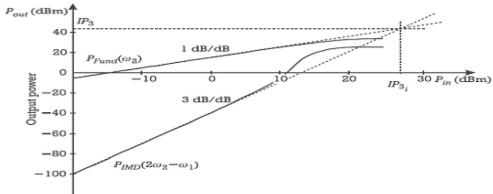
Output fundamental power per tone and distortion power in one IMD sideband for an equal amplitude two-tone excitation.
