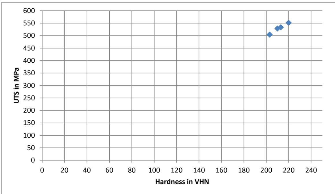
Figure 6:- Graph between hardness and UTS
