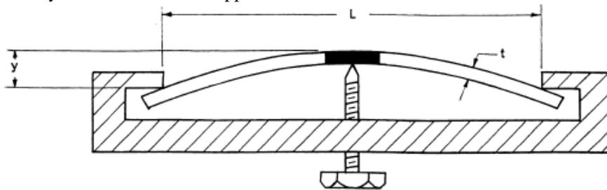
Figure 1:- Schematic of three-point-loaded, bent-beam test Apparatus [5]
