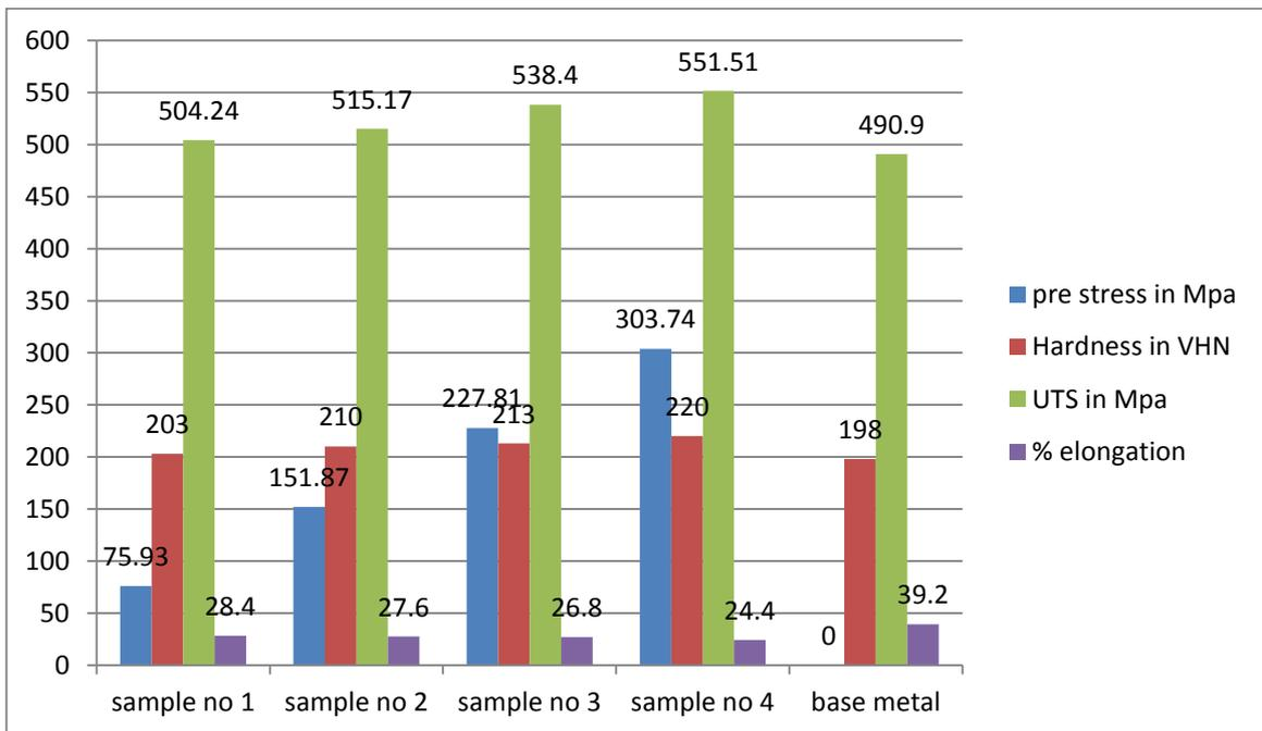
Figure 8:- Comparisons of properties between four samples and base metal
