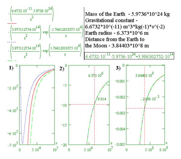
The first function has been known since the time of Newton. The two further functions are formed when in Newton's function we put an exponential factor in the form of  $\exp(-B/x)$  and  $\exp(B/X)$ . (In these two functions, the coefficient B=1.76612818375 and dimension of the coefficient B is m, or meter.)
