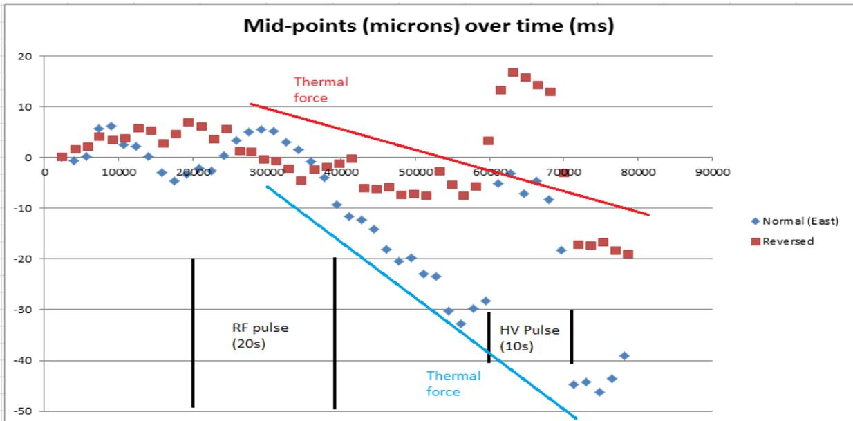
Figure 8. Spurious thermal forces depend on frustum orientation.
