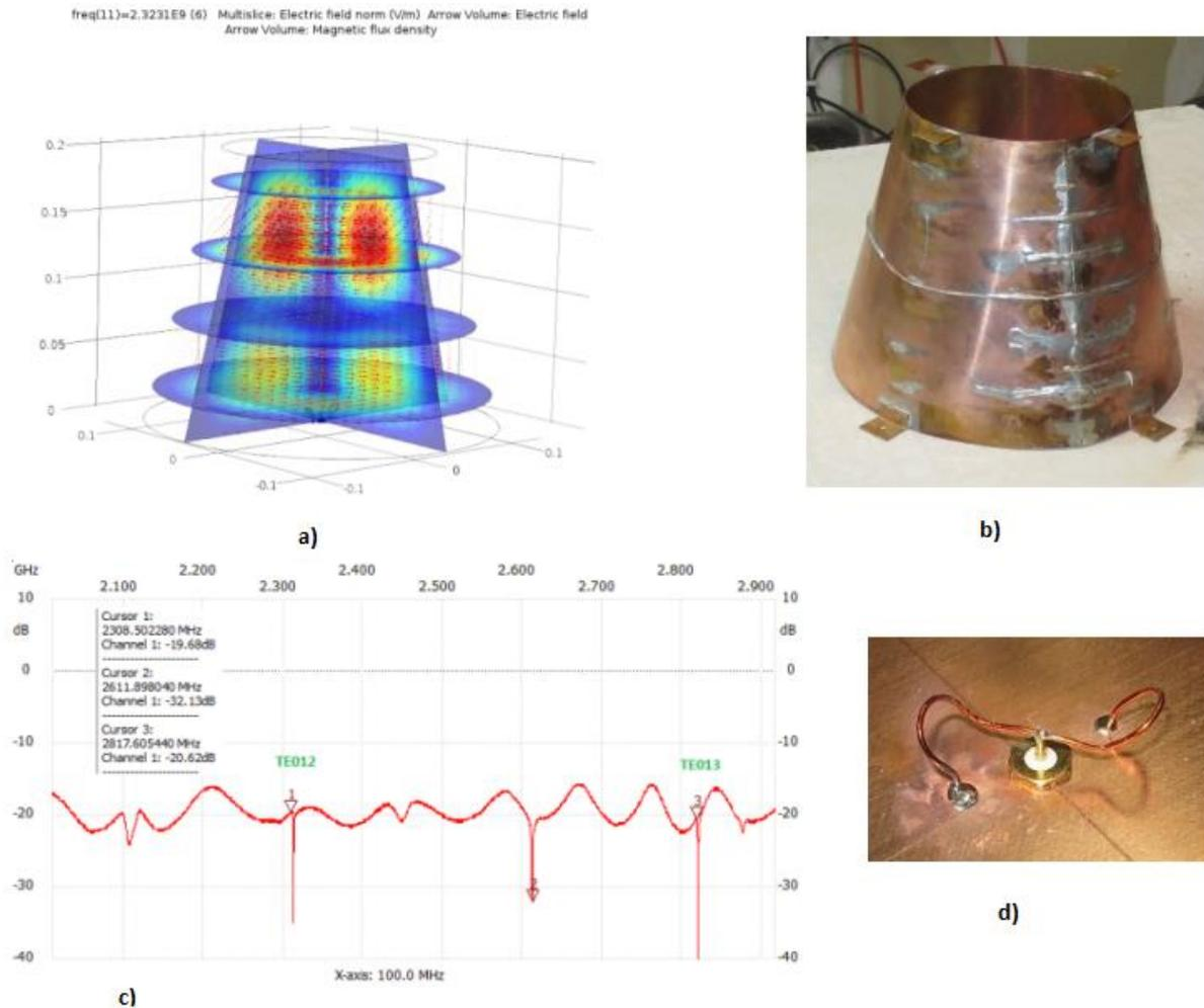
Figure 4. RF cavity. (a) COMSOL(c) simulation of TE<sub>012</sub> resonance mode. (b) Copper frustum as-built. (c) S<sub>11</sub> frequency scan using a -20 dB directional coupler. (d) Coax coupler on the big end plate.
