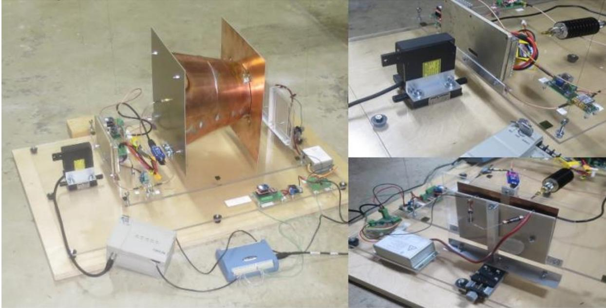
Figure 1. Test platform showing RF cavity, laser distance sensor and electrostatic attraction plates.
