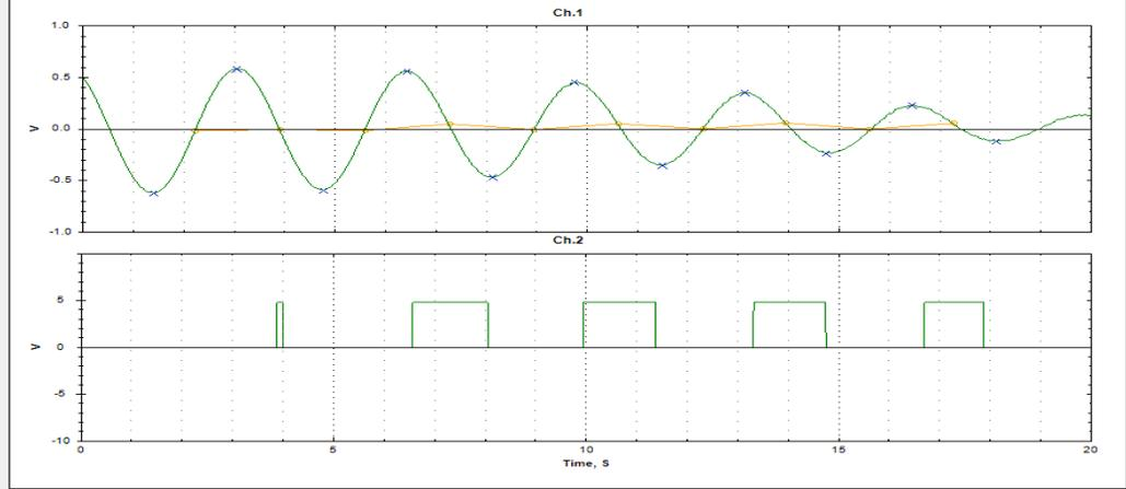
Ch1. Pendulum position (1V = 1000  $\mu\text{m}$ ) and mid-points of oscillation over time.
