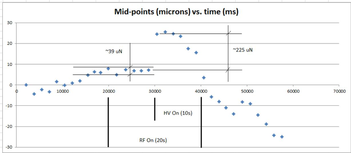
Figure 7. Low noise test run with electrostatic test pulse overlapping the RF pulse.
