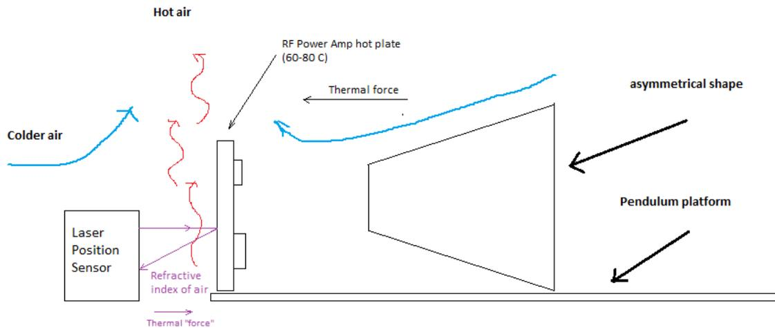
Figure 9. Potential sources of spurious thermal forces.
