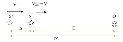
Now we apply the above general analysis to the specific case of moving source and stationary observer shown above. Consider a light source moving towards an observer that is at absolute rest. We want to show that the speed of light is independent of the speed of the source.
