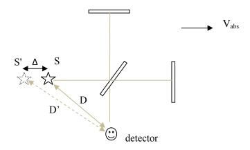
In the above diagram of Michelson-Morley experiment, the real source S has been replaced by an apparent source S'. Once we replace S with S', we assume the speed of light to be constant relative to S'. We may think of this as applying conventional emission theory to S'.
