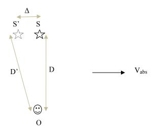
During the time interval that the light goes from S' to O, the source goes from S' to S.
