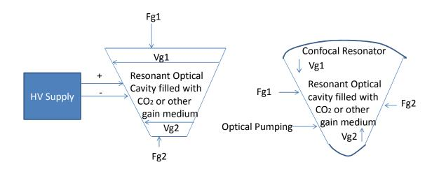
Figure 5. Increased Photon Density and Thrust Using an Electrical or Optically pumped LASER
