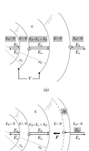
Fig.2. - The displacement,  $\Delta x$ , of the electric field,  $E_b$ , into the outer shell. Thus, in the region with thickness  $\Delta x$  the intensity of the electric field is not null but equal to  $E_b$ .
