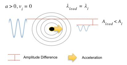
Fig. 6.3 - Force on Particle at Rest
