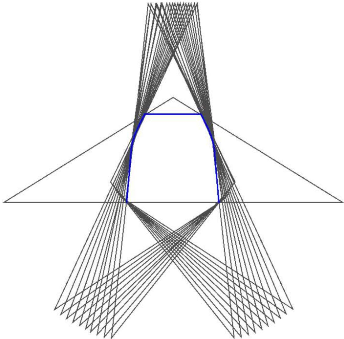
For the next phase the path is constructed from similar segments to the truncated caliper including circular arcs between two straight lines on each arm. However, the apex of the triangle is no longer pinned to the endpoint of the curve to form these arcs. Instead the triangle moves so that the end point slides along one of the edges of the triangle while the other two edges slide round the arcs.
