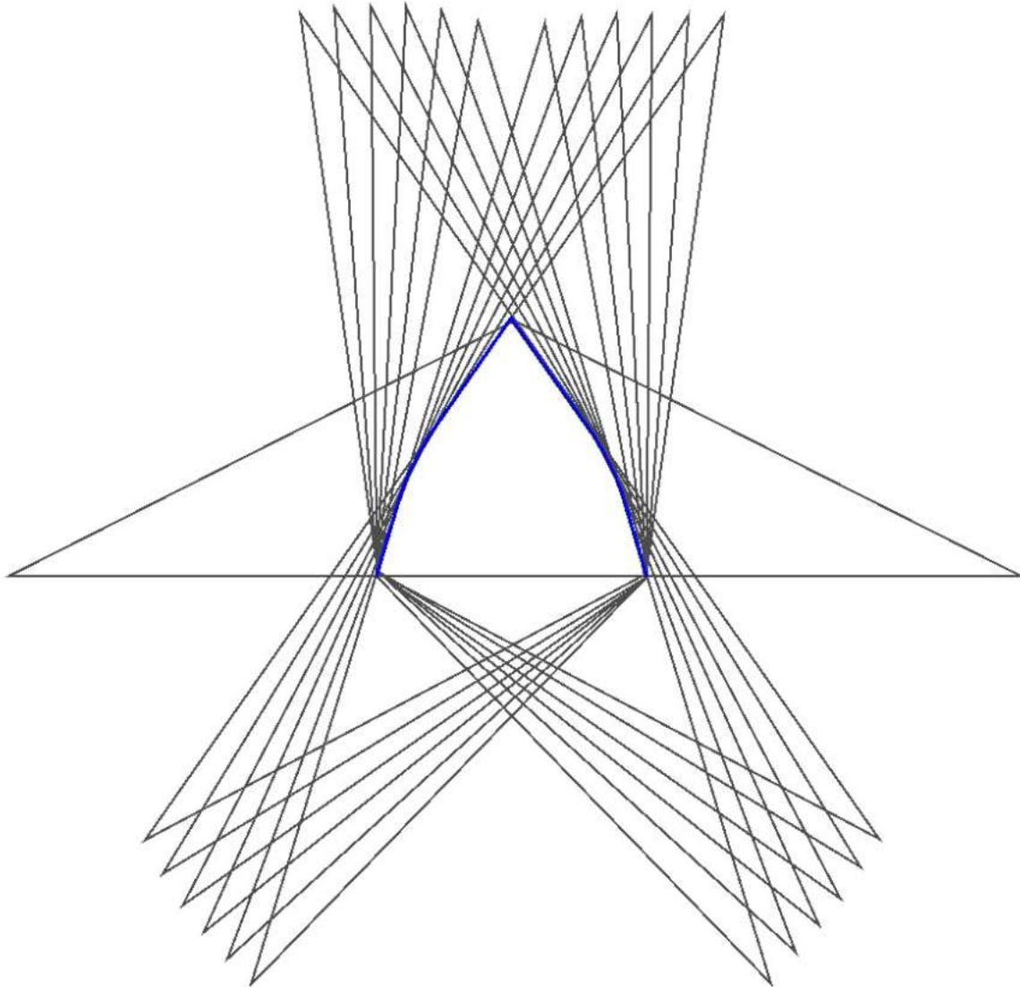
Zalgaller's Caliper (also known as the broadworm) is the solution to Bellman's problem for a long thin strip. It has two arms each consisting of two straight lines joined smoothly in the middle by a circular arc. The two arms meet at a sharp apex at an angle of nearly 70 degrees. The caliper also fits comfortably inside an isosceles triangle for small base angles  $T$ , so it also works as an escape path, but for what angles is it the shortest escape path?
