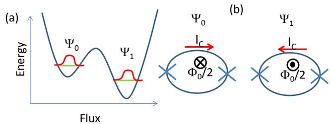
Fig. 4. SQUID as Flux Qubit. (a) Double-well potential energy of bistable SQUID, showing quantized energy levels and distributed quantum waves. (b) Configurations of currents in two classical states, which may be combined in superpositions for the flux qubit.
