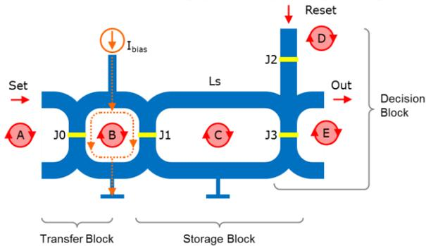
Fig. 3. Schematic of flip-flop in Rapid-single-flux-quantum (RSFQ) logic, a classical computing system using Josephson junctions and SFQ voltage pulses (figure from [6]).
