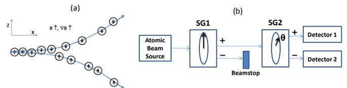
Fig. 7. Stern-Gerlach experiments using magnetic fields to separate atomic beam components of different spin. (a) Mixed beam of spin-up and spin-down atoms separated by inhomogeneous field. (b) Block diagram of two-stage Stern-Gerlach experiment to test for spin superposition. This standard textbook thought-experiment has never actually been carried out.
