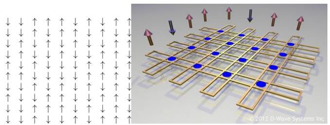
Fig. 5. Analog Simulated Annealing Processor. Left, 2D Ising Model, consisting of array of coupled atomic spins. Right, array of inductively coupled SQUIDs, functioning as flux qubits, designed to map onto spins in the Ising Model (figure from [28]). At sufficiently low temperature, an annealing processor is expected to cross over from thermal annealing to quantum annealing.
