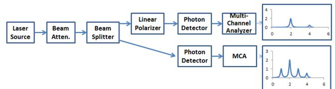
Fig. 8. Block diagram of experiment to test for linearly polarized single photons. New superconducting photon detectors have high quantum efficiency and energy resolution.
