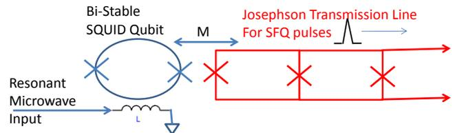
Fig. 9. Block diagram of experiment to test for superposition in flux qubit. Flux changes in the loop can be measured by observing SFQ pulses coupled out, while avoiding environmental loading and noise.
